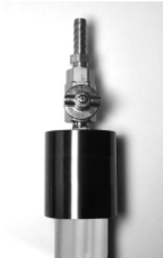
Figure 9-4. Leak check/flow adapter.
